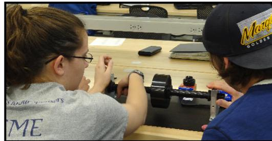
Figure 7: Investigating bearing operation in Experiment 6.
